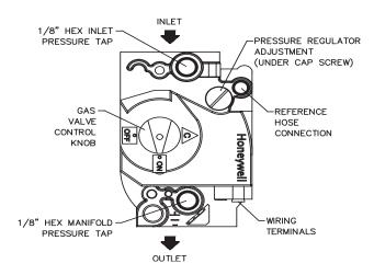
FIG. 45 Combination Gas Valve
